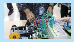
One of the main focuses of this lab is to connect the theoretical background taught in the Control System course with the realities of physical hardware and simulation. The laboratory is well equipped with digital oscilloscopes, LabVIEW, MATLAB/Simulink software and a LJ MS15 DC Motor Control Module.
